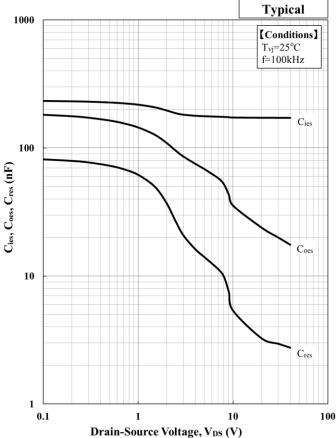
Capacitance vs. Drain - Source Voltage
