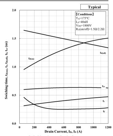
Switching time vs. Drain Current
