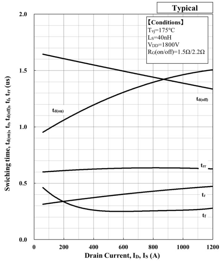
Switching time vs. Drain Current
